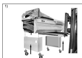
Lift the machine from the pallet by using a fork lift truck. Fit the 2 legs using the 4 screws taken from the plates plus the other 4 supplied in the kit.
